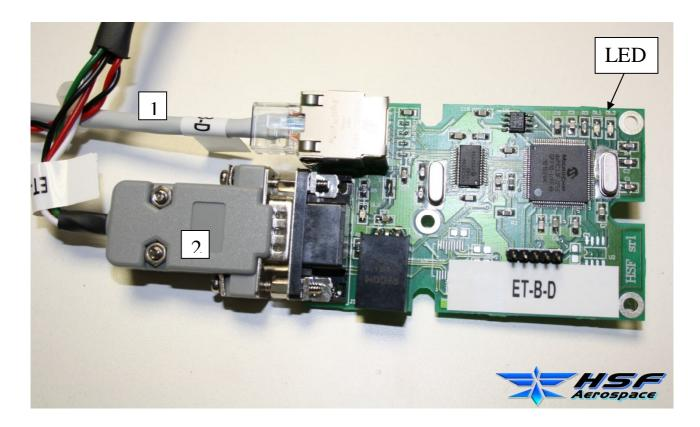
This is device that allows the communication between the boards and the host , using the cable'lan .
