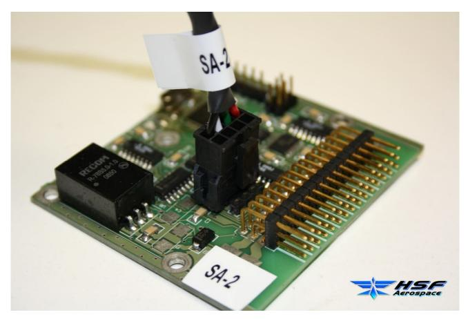
In this board must be connect the cable's data and powered like in picture. After can be connect all of the following cables :
